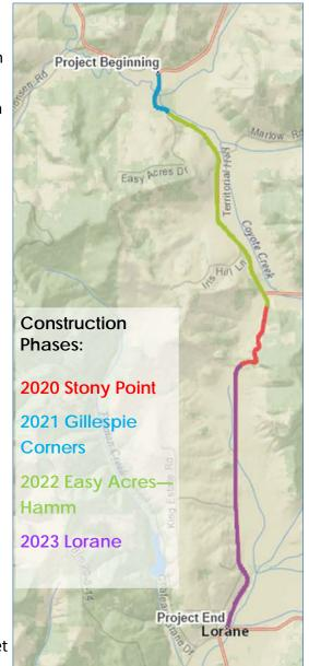
**Next Steps:** The County is in the process of designing Phase 2 of the project — improving the road at Gillespie Corners. Planned improvements include raising and widening the road and bridges to accommodate six-foot-wide shoulders, and adding an overflow structure to prevent roadway flooding during heavy rains. Construction of Phase 2 is scheduled for 2021.
